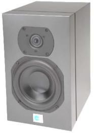
The Sat 6D features both XLR Analog inputs and AES/ EBU Digital inputs. The DSP crossover filters are derived using Blue Sky proprietary BOO optimization software. The Digital circuitry features FR4 6-layer circuit boards, Burr-Brown 192kHz/24 Bit A/D & 192 kHz/24 D/A, and Cirrus Logic Digital receiver and sample rate convertor. In addition, the Sat 6D has a "Pure-Digital" mode for 48 kHz and 96 kHz operation, where the native input from the AES/EBU receiver is sent straight to the DAC.
