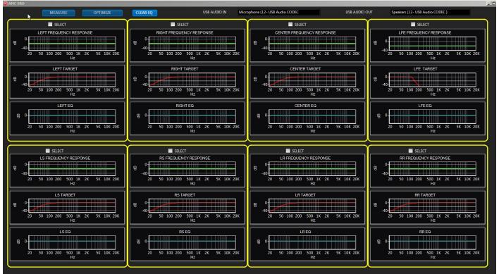
This screen shows the current state of the EQ, target filters, measured frequency response and corrected frequency response of all the channels. Clicking on any of the small graphs will open up a larger graph.
