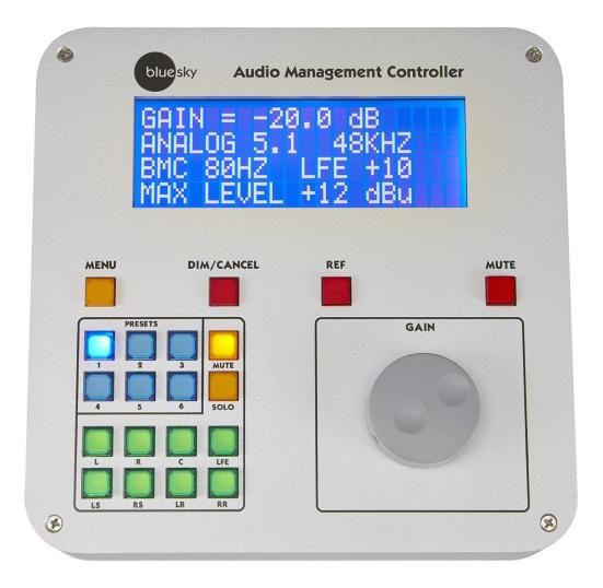
**GAIN** – changes the system gain in 1.0 dB increments . Also used to scroll through the menus and change parameters.
